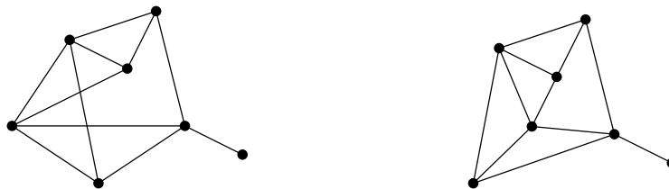
Figure 2.2: A planar graph (left) and a plane drawing of it (right).
