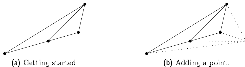
Figure 5.2: Constructing the scan triangulation of P .
