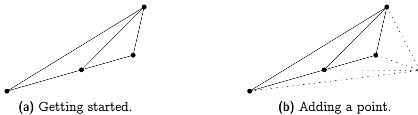
Figure 5.2: Constructing the scan triangulation of P .
